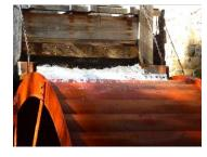
• 41.1 cubic feet of water per minute pouring into the wheel produces 1 horsepower.
